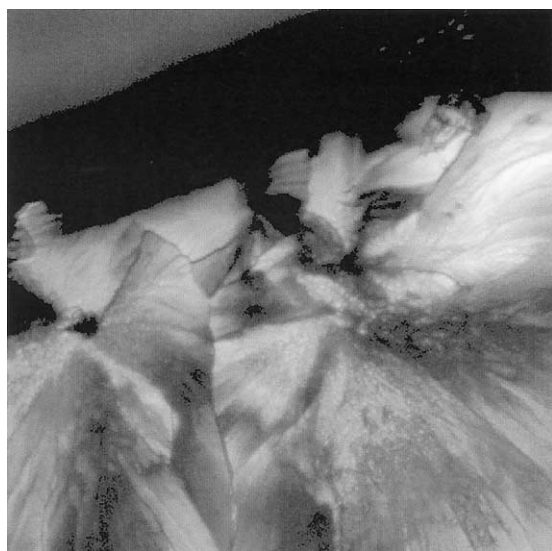
Fig. 4. The crystalline region on a 7-day-old felodipine sample observed by polarizing microscopy under crossed polarizers (magnification 20 times). Note that the glassy region is dark and the crystallized region is birefringent.
